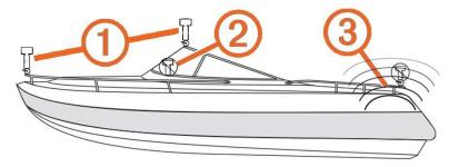
• The antenna should not be mounted where it is shaded by the superstructure of the boat ②, a radome antenna, or the mast.
